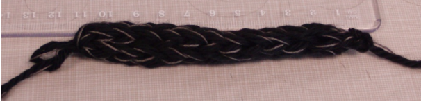
Fig. 10. A knit stretch sensor at slack length. The conductive yarn is silver, the actuator yarn is black. Units on the ruler are centimeters.
