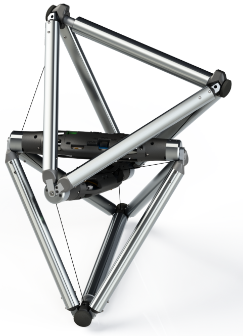
Fig. 1. Render of the DuCTTv2 Prototype. A system of eight independently actuated cables connect two nested tetrahedra to produce complex high degree of freedom motions.
