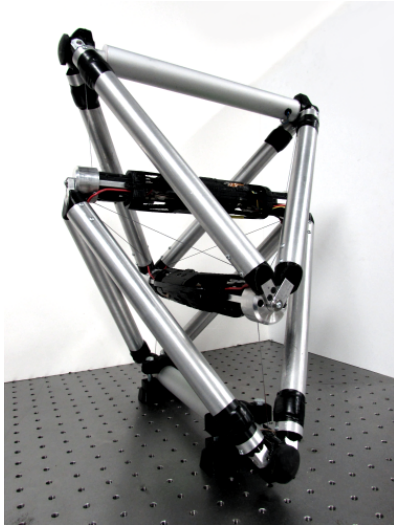
Fig. 2. Image of the DuCTTv2 hardware prototype. The topmost and bottommost rods are linear actuators used for wedging between duct walls. The four hollow vertical aluminum rods of each tetrahedron house batteries and cabling. The two central rods encased in black plastic each house all the needed control circuitry and four BLDC motors for cable actuation.
