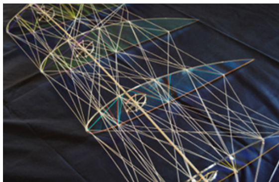
Figure 1.1: Tensegrity wing structure demonstration hardware made by Skelton [1]
