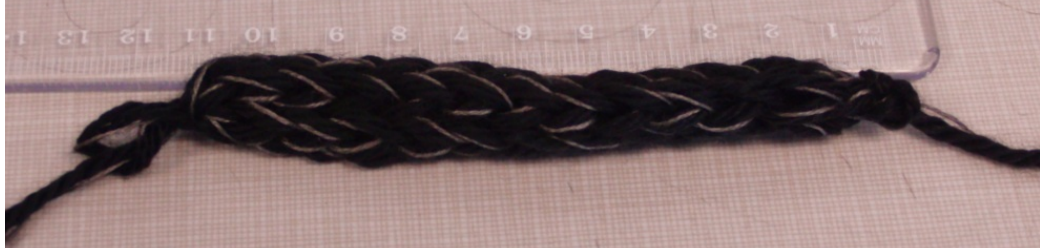
Figure 7.2: A knit stretch sensor at slack length. The conductive yarn is silver, the actuator yarn is black. Units on the ruler are centimeters. From [Tietz et al., 2013].
