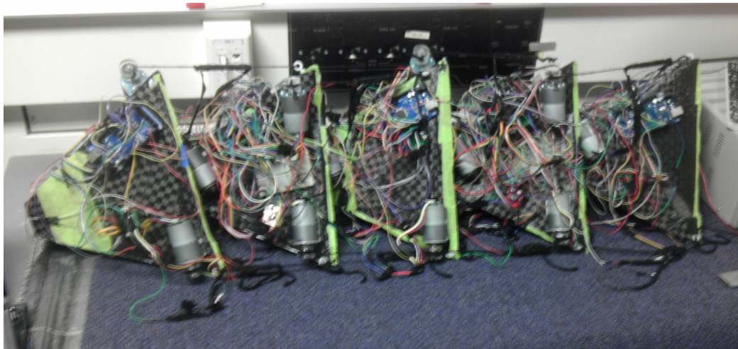
Figure 7.5: The five segment version of the Carbon Fiber spine. Ultimately the forces required for movement of this spine were beyond the strength of the knit stretch sensors.
