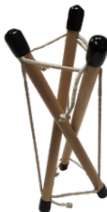
Fig. 2.1: 3-rod prism tensegrity structure
