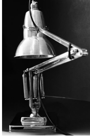
Figure 2.6: Anglepoise lamp: An example of a balanced arm design with zero stiffness mechanisms with tensioned springs. This mechanism was first patented by George Carwardine in the 1930s [25].
