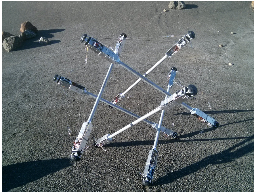
Figure 3.1: SUPERball, fully assembled, in the NASA Ames Research Center Roverscape.
